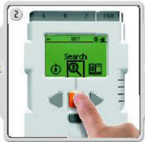
2 Select the Search icon to search for other Bluetooth devices. Your NXT will automatically search for Bluetooth devices.
