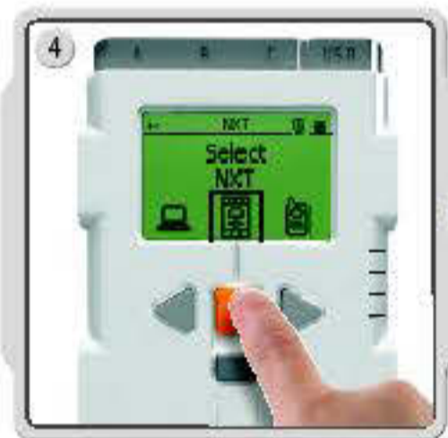
4 Select the device you want to connect to. Remember that you can give each NXT a unique name – see Naming the NXT on page 21.
