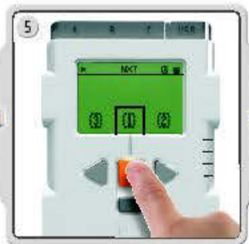
5 Select which of the three lines of communication you want the connection to be on (1, 2 or 3). You can connect your NXT to three different devices at the same time.
