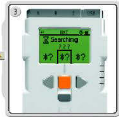
3 Depending on how many devices are detected in the area, a list will pop up on the NXT's display after a few seconds.
